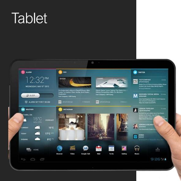
▶ a thin, flat <u>mobile computer</u> with a touchscreen display, which is usually in color, processing circuitry, and a rechargeable <u>battery</u> in a single device. Tablets often come equipped with sensors, including digital cameras, a <u>microphone</u>, and an <u>accelerometer</u>, so that images on screens are always displayed upright. The touchscreen display uses the recognition of finger or stylus gestures to replace the mouse, trackpad and keyboard used in laptops.
