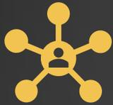
An Adhoc network is a peer-to-peer based network that doesn't use a central resource (Access Point) to manage the network connections and structure.
